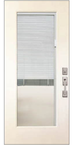
Full Lite Blinds 6-8 2-6 / 2-8 / 3-0 wide Value Series patio door flush glazed with BBG Blinds between glass, Smooth door skin shown with Shoji White paint. Clear IG glass is 22" x 64" in 2-8 and 3-0 doors, and 20" x 64" in 2-6 door.
